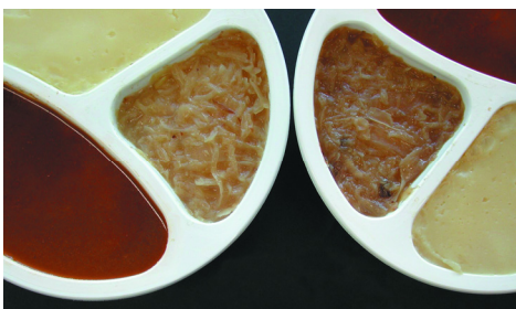
Color changes in stored ready meals: Left: Packaging with O 2 -scavenger Right: Packaging without O 2 -scavenger
